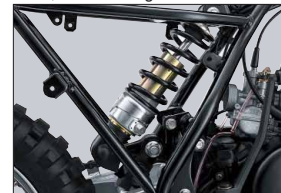
Rear suspension with mono-shock absorber
