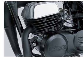
79 cc, 2-stroke engine
