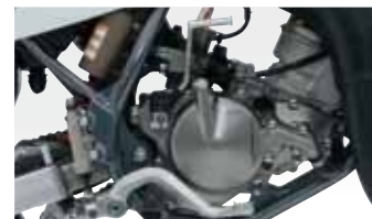
84.7cm 3 2-stroke engine
